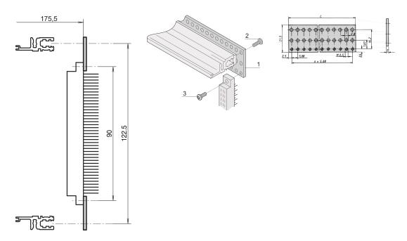
Perforated flat rail for connector mounting i.a.w. EN 60603-2 and DIN 41612, on VT horizontal rails.
