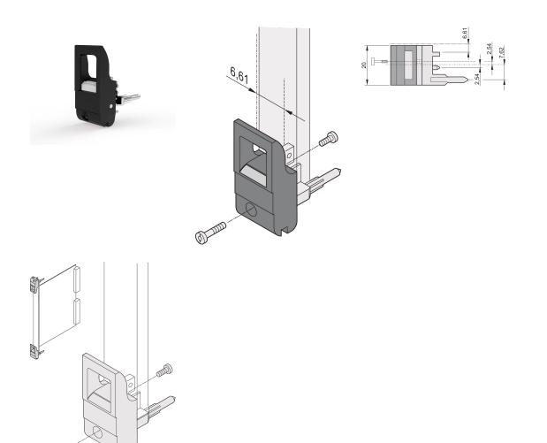
The inserter/extractor handle, type IET in accordance with IEEE 1101.10. 0,1" offset. Two of these handles can overcome a single lever force of 700 N (per pair).
