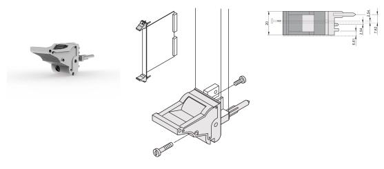
The inserter/extractor handle, type IEL in accordance with IEEE 1101.10. 0,1" offset Two of these handles can overcome a single lever force of 700 N (per pair).
