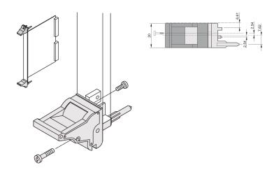
The inserter/extractor handle, type IEL in accordance with IEEE 1101.10. 0,1" offset Two of these handles can overcome a single lever force of 700N (per pair).
