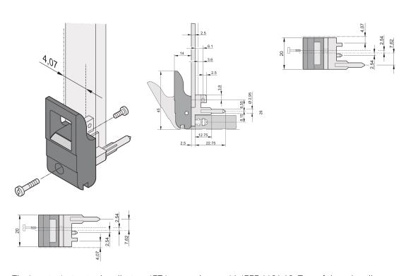
The inserter/extractor handle, type IET in accordance with IEEE 1101.10. Two of these handles can overcome a single lever force of 700 N (per pair).
