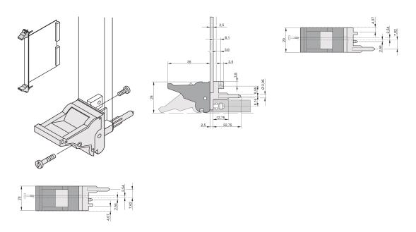
The inserter/extractor handle, type IEL in accordance with IEEE 1101.10. Two of these handles can overcome a single lever force of 700N (per pair).
