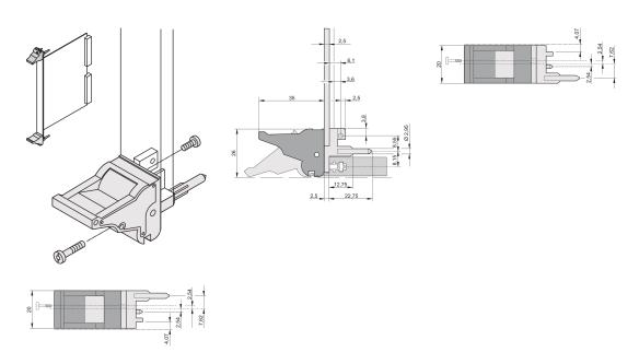
The inserter/extractor handle, type IEL in accordance with IEEE 1101.10. Two of these handles can overcome a single lever force of 700N (per pair).
