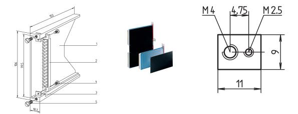
Accepts PCBs in Euroboard format, 100 x 160 mm. Plastic material PBT.
