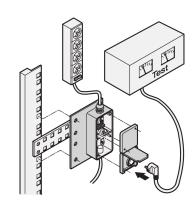
Distribution box is used to house PDUs which safely distribute electricity from power source to devices in a circuit.
