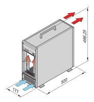
VME64 tower system for 7 VME64x boards 6 U, 160 mm. The power for the system is supplied by a open frame power supply. A fan control module monitors the fans, the temperature and voltage.
