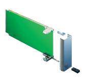
Handle mechanism AMC.0 Rev. 2.0, MTCA.1 and MTCA.4 Modules.
