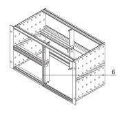
The 2 HP wide front panel covers an open slot. The non-shielded version can be fixed with screws and washers. Due to the 2 HP width, no sleeves can be used.
