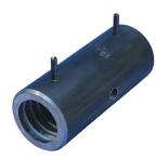
The side fill horizontal T-Series sleeve has vent holes located 90 degrees from the tap hole to facilitate side fill installations when the interferences of the structure will not allow top filling. The vent holes are added to horizontal sleeves to reduce air entrapment and help ensure proper filling of the sleeve.
