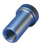
One-piece flange couplers are ideal for eliminating protruding dowel bars in segmental pour applications. The flange side of the coupler is typically tack or seal welded to cast-in-place structural steel walls commonly found in most modern nuclear reactor designs.
