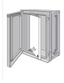
Swing-Out Panel installs into Ultrx fiberglass enclosures. The front-mounted swing panel complements window-door units and is suited for any application requiring a display of gauges, dials or any type of control equipment monitor. Easy installation; no drilling required. Fully adjustable front to rear. Front mounting position is approximately 140mm (5.5 inch) back on 400mm enclosures. Panel, mounting hardware and instruction manual included.
