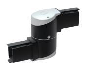
Syspend 281-Max Intermediate Joint to join two horizontal tubes together for a longer run. Arm can be rotated or turned 300 degrees. Includes safety stop and maintenance-free bearing. Use of the Intermediate Joint reduces the system load capacity to 179 lb. (81.2 kg) at 3.3 ft. (1 m).
