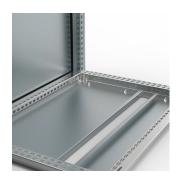
A split bottom plate offers a flexible cabling solution and eliminates the need for individual cable glands. The protection degree is maintained by using a separate gasket.
