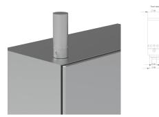
This high temperature Vortex cooler, HT, with a IP 66 protection degree, is easy to install, has no moving parts, and is maintenance free. In addition to cooling, it also reduces the relative humidity within the enclosure it is mounted on. This Vortex cooler is an ideal solution to prevent overheating within the enclosure in environments up to 93°C, for example in a steel mill.
