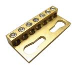
nVent ERIFLEX Connecting, Earthing and Neutral Busbars are used to connect several earthing conductors within a panel and can be used in a variety of different applications including switchgear and control equipment, electrical equipment, for wind and solar power generation and in data centers. This Universal Connecting Bar can be used as a 450A current rating IEC for power distribution.
