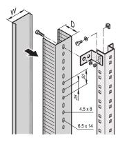
Cable ducting in side and rear cabinet areas and mounting on cabinet uprights, depth members or C-profiles.
