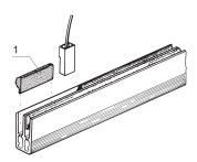
Contact Protection for Busbar for electrical insulation.
