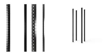
Slide mout with adjustable increments. Assembly in 600 mm wide cabinets directly on the frame. At 800 mm width adapter bracket for reduced width is neccessary, for partial-height mounting depth members are necessary.
