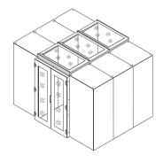
Blanking panels for different aisle containment heights to avoid air leakage at aisle swing doors.
