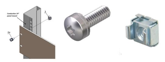
For standard grounding use a grounding nut and washer on at least one attachment point.
