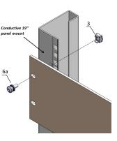
Accesory parts like screws, washer and nuts enable the mounting of 19" accessories.
