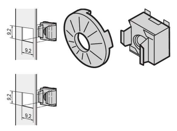
Cage nuts permit range of choice of nut and bolts sizes and easily replaced unlike pre-threaded holes. Cage nuts are easy to use on materials too thin or soft to be threaded.
