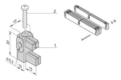
Mounting Brackets for Busbars or Busbar Modules are load circuit isolated mounting units for grounding rails. There may be adapters with assigned current ratings which supply the load current to loadfeeders through wire connections.
