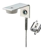
The nVent CADDY Speed Link Light Pack with Nail Gun Bracket includes a precut length of 1mm wire rope riveted to an angle bracket designed for direct fastening together with an ultra-low-profile locking device. Contractors can quickly and safely install it to the concrete ceiling using a wide range of nail guns to support and secure lighting and signage.
