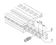
Perforated strip out of 1mm Aluminum for centering shielded plug-in units.
