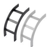
The Ladder Rack Curved Sections provide a vertical change in direction. They are made of 1-1/2 inch x 3/8 inch (38 mm x 8 mm) tubular steel with a painted or plated finish. Cross members are welded on the inside (inside bends) or outside (outside bends) of the section. They connect to straight section with butt-splice kits. They are also designed for category 5e, 6, 6A and fiber optic cable.
