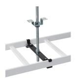
The Cable Runway Center Support Kit is a threaded rod and bracket that supports the center of ladder rack from a ceiling. The kit includes a heavy-duty ladder rack cross member, two mounting brackets, two #12-24 screws, a 5/8-inch threaded rod, a protected sleeve and four 5/8-inch nuts. Supports should be used at least every 5 feet (1.5 m).
