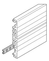
Adapter / Mounting opportunity for fixing of any compents with M3 screws. The threaded insert is slid into the groove of the inside of the side panel.
