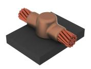
nVent ERICO Cadweld Cathodic Connections are the preferred method of exothermically welding cathodic protection anode leads to pipes (steel or cast iron), tanks, and other structures. Cathodic protection systems are designed to prevent galvanic corrosion along a pipeline or in various structures. nVent ERICO Cadweld Cathodic Connections use a special welding material alloy to minimize heat effect on the steel, which is especially important on thin wall and high stress pipes.
