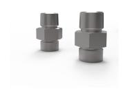
This plumbing adapther is a male-male fitting with 1" BSPP flat seal thread on one end and 1" NPT on the other. It adapts the BSP style 1" hoses for installation in US style NPT chilled water facilities.
