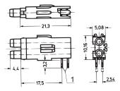
Double test sockets for mounting plane 1 and 2, short and long type.
