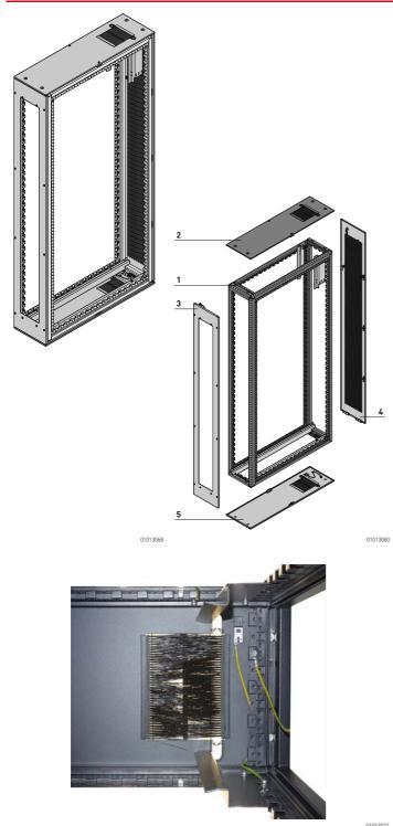
Water enters via brush strips; lateral cable ducting for power/data cables
