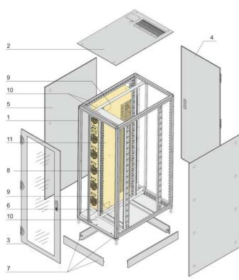
Cabinet with air/water heat exchanger with cooling capacity of 34 kW
