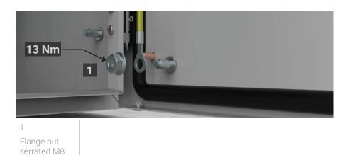
13 Nm 13 Nm 6 2 5 4 3 1 2 3 5 6 4 1 Earthing Plain Hexagon Plain Nut M8 Nut M8 screw washer washer M8 washer M8x30 Μ8 Μ8
