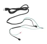
Use to power 120 VAC Compact Axial Fans; replaces existing supplied power cord. Fan cord includes inline thermostat. Fan(s) will turn on when the inline thermostat reaches 86F (30C). Fan(s) will run only when temperature is above 86F (30C). Use with 110-120 VAC fans with power cords only. One or two fans can be used with power cord.
