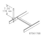
The Cable Runway Retaining Post Kit provides extra ladder rack capacity. The retaining post mounts onto the rack side stringer. The post is made of an unthreaded 1/2-inch tube. The kit includes post cap and mounting hardware.
