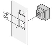
Square nuts have higher contact surface and dont get rounded off unlike hex nuts. For precise, anti-twist secure mounting without clearance, use square nuts.
