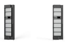
The new rear door cooling units from nVent are offered in a range of standard sizes for use with 42U, 47U, in both 600mm and 800mm widths (other sizes available on request). The coolers themselves are 250mm deep, with a dry weight of 140Kg. One of the features of rear door coolers is they are compact and do not require any additional floor space or ceiling headroom – in fact, their use can free up white space as CRAH units and other room cooling equipment may be eliminated from the data centre.
