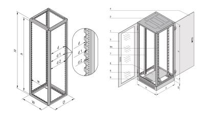
Basic rack to support cabling and networking equipment. Cooling via convection or top cover fans.
