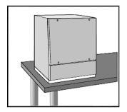
Base closes off open bottom of ProLine Sloped-Front HMI Enclosures that are table-top mounted or suspended from overhead. Base includes a ground stud. Foam-in-place gasket assures a water-tight and dust-tight seal. A top support bracket can be installed inside a 600-mm wide base for reinforcement when a Compact Series 4 System 80 is attached from below.
