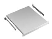
The Rack-Mount Adjustable Shelf mounts to the front surface of front and back rack angles. The adjustable shelf support brackets are clear-plated 12 gauge steel and adjustable to fit multiple-depth enclosures or rack angle placement. There are both solid and vented models available. They fit 19- or 23-inch rack spacing and require only 1U of rack space. Please note the load rating is for 150 lb. (68 kg).
