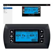
The Disply unit allows for local configuration, comissioning and monitoring of the RackChiller Rear Door. It encorporates an LCD panel display and 6 function keys. It installs directly to the cooler's external panel, and connects to the pre-wired cabling within the unit.
