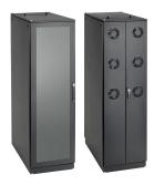
The ProLine FloTek FD Server Cabinet uses the cooling power of two banks of independently-powered fans in the back of the cabinet and an integral front floor duct to direct air into server intakes when positioned over a cutout in a raised data center floor. The cabinet air inlet requires alignment with a floor cutout so blocking plates can direct cool air from the floor plenum across the front of the equipment.
