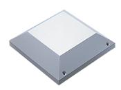
Vents fit on standard ProLine top with vent cutout or can be field-installed on any ProLine solid top. The Pagoda Vent features an integral centrifugal blower mounted in a housing that includes a drip-proof removable hood, wire mesh finger guard, perimeter gasket and terminal block. Electromagnetic-compatible (EMC) Pagoda Vents include a conductive screen, conductive gasket, line filter and 6-ft. power cord with stripped leads.
