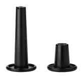
The Cable Spools organize and direct cable while maintaining a minimum cable radius. They fasten easily to Heavy Duty or Seismic racks with a single screw. The spools can also be used with patch panels, grid straps or plywood walls for general cable management. The necessary mounting screws are included.
