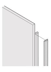
The textile EMC gaskets are inserted into a slot on the right hand side of the U-shaped front panels. The gaskets are glued to the front panel.
