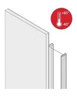
The textile EMC gaskets are inserted into a slot on the right hand side of the U-shaped front panels. The gaskets are glued to the front panel. For an expanded temperature range up to  $+85^{\circ}$ C.
